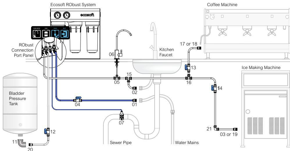
Some of the fittings shown on the diagram come from RObust package. These fittings can be used interchangeably or together with the fittings from RObust connection fitting pack when it's necessary to connect more than one appliance with  $\frac{3}{8}$ " or  $\frac{1}{2}$ " female thread ports or a  $\frac{3}{4}$ " pressure tank.
